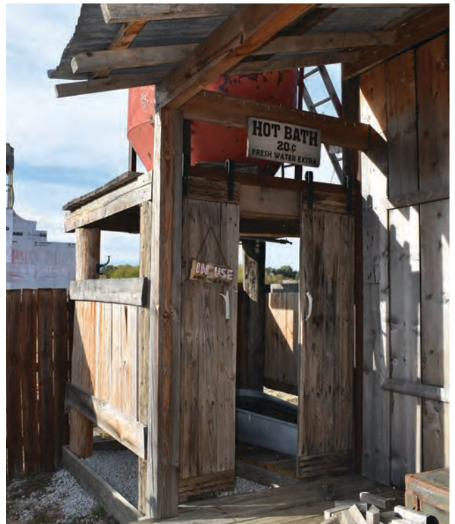
A bathhouse that would have been available for public use. Rainwater would be held in the red water tank and used for the showers.
